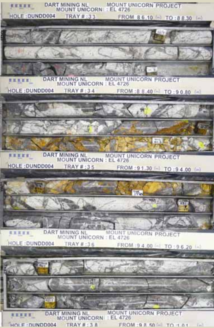
Above: Quartz vein stockwork with multiple cross-cutting generations (DUN004)
