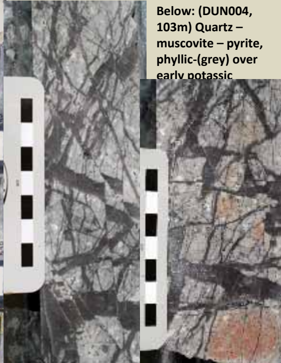
Above: Quartz vein stockwork with multiple cross-cutting generations (DUN004)
